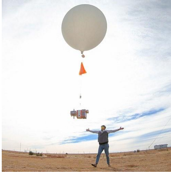
Figure 4. Example launch of a small (weather) balloon launch with a payload of in situ instruments for ozone, water vapor, and aerosol measurements. These balloons reach a maximum altitude of 30 km (100,000 ft) and telemeter data to the ground during flight since many payloads are not recovered. Source: NOAA Chemical Sciences Laboratory.
