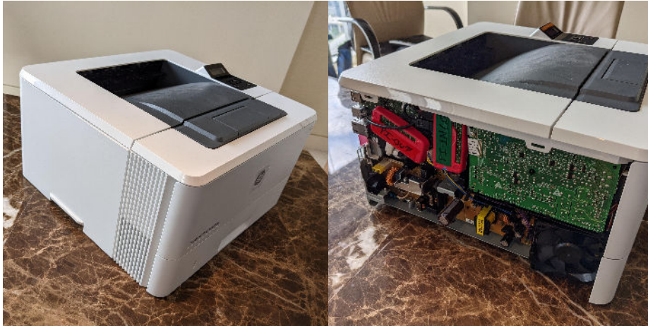
Figure 4: Demonstration Malicious Hardware. I developed a hardware-based attack that modifies data sent from the ICX to the printer, altering ballot QR codes to change recorded votes. The attack device (the two red modules seen in the right photo) is completely hidden inside the printer's plastic housing. Similar malicious hardware could be added in the supply-chain or while in storage.
